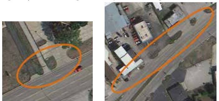
Figure 6 | These two images highlight areas with a high number of access points with very little separation. This is problematic throughout this segment of the corridor making traffic conflicts likely.
